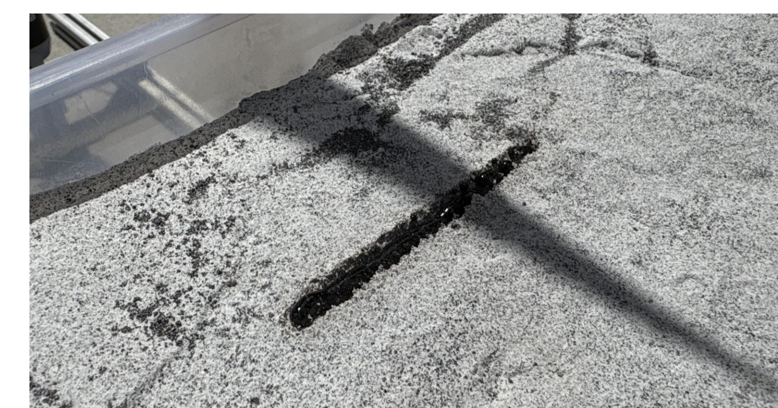
Fig. 8: Straight line sintered sample.
